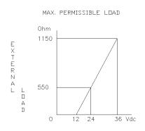
The maximum permissible load (Ri max.) in case of 24 Vdc is 550  $\Omega$  (Ohm).
