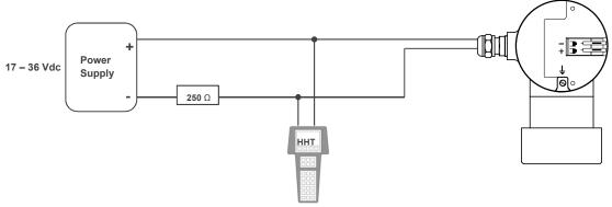
Option 2: HART <sup>®</sup> Handheld terminal connected across the loop resistor.
